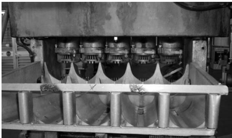
Figure 8.15 Cups of the FMC Inline Juice Extractor. (Courtesy of the Department of Biotechnology and Food Engineering, Technion, I.I.T.)
