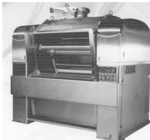
Figure 7.9 Horizontal dough mixer
