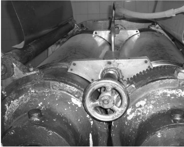
Figure 22.32 Drum dryer. (Courtesy of the Dept. of Biotechnology and Food Engineering, Technion, I.I.T.)
