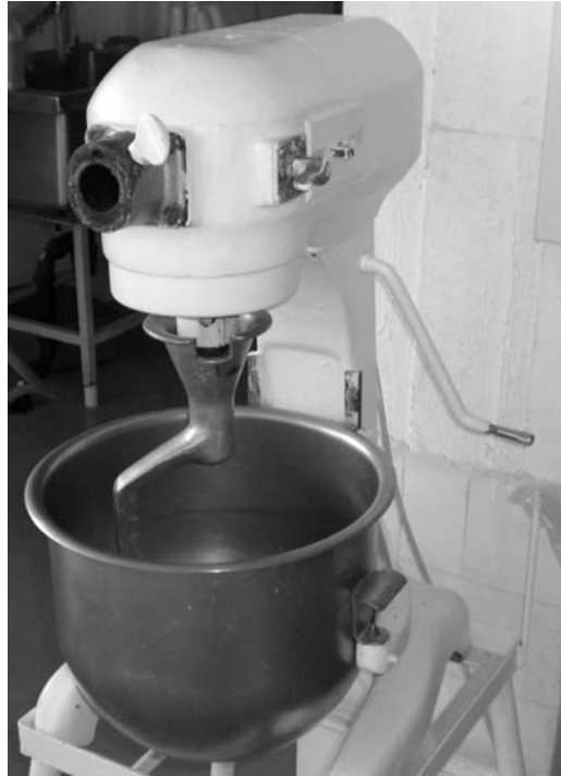
Figure 7.8 Planetary mixer. (Courtesy of the Department of Biotech. and Food Engineering, Technion)
