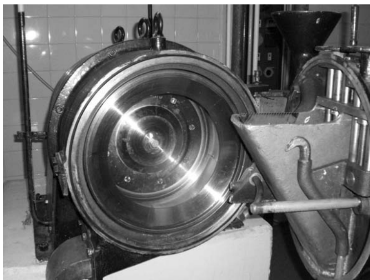
Figure 8.13 Vertical basket centrifuge showing scoop and scraper assembly. (Courtesy of the Department of Biotechnology and Food Engineering, Technion, I.I.T.)
