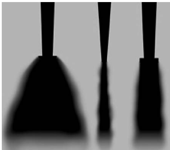
Figure 22.27 Different types of sprays obtained by ultrasonic atomization. (Courtesy of SonoTek Corporation)
