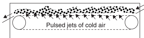
Figure 20.8 Principle of fluidized bed (IQF) freezing
